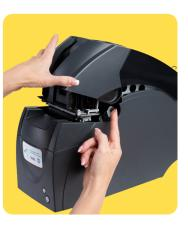
3 Load the paper roll into the Printer with the BCLC colour bar on the right. The Lotto Paper should come up from underneath the roll.
