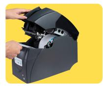
Press down firmly and close the Printer door. The cutter will automatically trim the paper.
